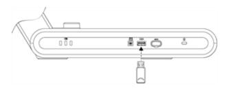
Then, using the remote control or document camera's control panel, press the **Capture** button to save an image, or press the or **Record** button to start recording video. Press the **Record** button again to stop recording. When you are ready to view the files, connect the USB drive to a computer or interactive display.
