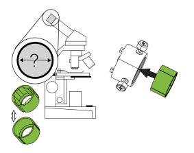
2. Attach the microscope adapter to the document camera and tighten the three bolts until the adapter is secured.
