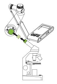
4. Turn the microscope adapter counterclockwise to line up the arrows and lock the microscope adapter in place.
