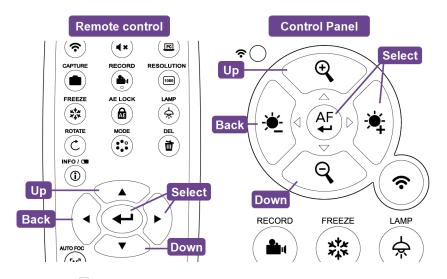
Press **Info** (1) on the control panel or remote control to exit the OSD menu.
